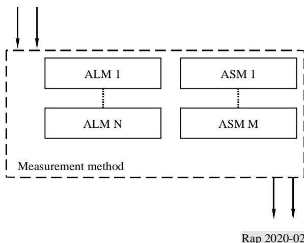
The proposed generic representation at entrance control point and final control one is the measurement structure shown hereafter. ALM and ASM are respectively the algorithmic and the associated modules composing the measurement method. The Indexes N and N' indicate that the module is located at entrance control for N or at final control measurement point for N'.
