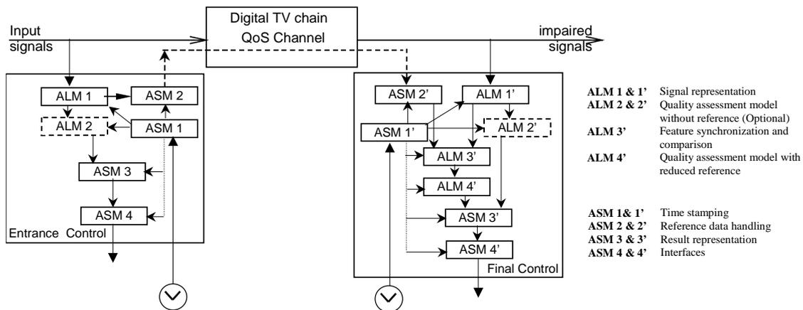
Figure 2: Detailed structure of the generic measurement method
