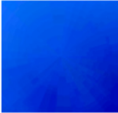
Figure 5. Example of zoom on radial blocking pattern in a portion of viewport corresponding to a portion of equirectangular frame affected by classical blocking artifacts due to block-based lossy compression.
