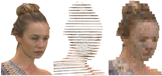
Figure 2. Point cloud compression results using the anchor software [2] at 13 Mbit/s: Original, decoded point cloud (geometry subsampled), decoded point cloud rendered with larger point size.
