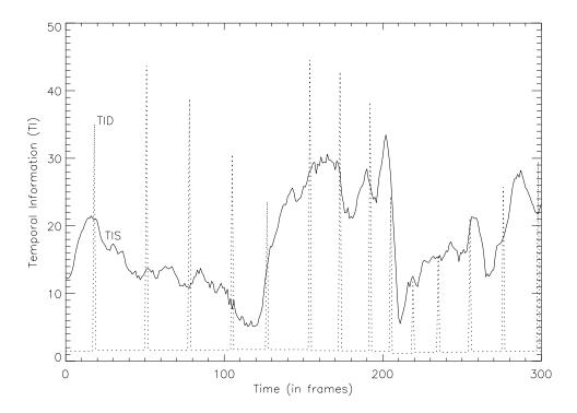
Figure 2 Plot Demonstrating Low Frame Rate HRC
