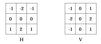
Figure 2 Horizontal and Vertical Edge Filters
