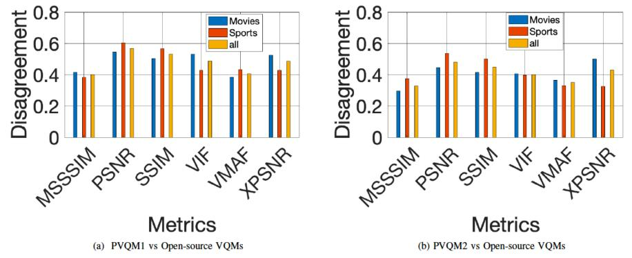
Fig. 8. Evaluating the fraction of PVSs on which the PVQMs disagree with each open-source VQM. The analysis indicates that the PSNR and SSIM are a bit more likely to measure a quality that would be perceptually different than that indicated by the PVQMs especially on Sports content.
