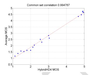
Figure 1. Scatter plot for the limited HD4 common set compared with the mean value obtained for the common set of the all experiments.
