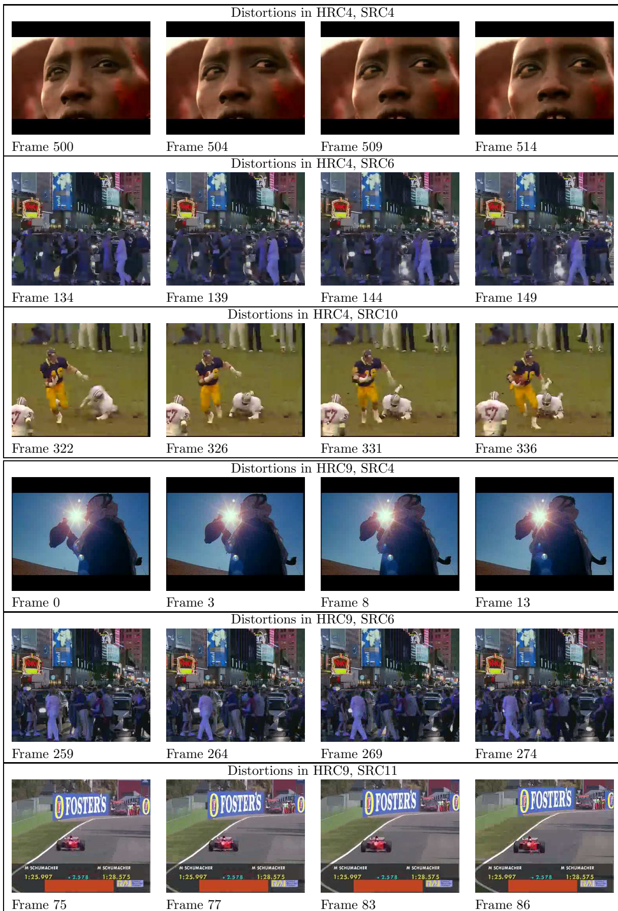
Figure 4.11: Typical distortion of H.264 (HRC4) and MPEG-4 (HRC9)
